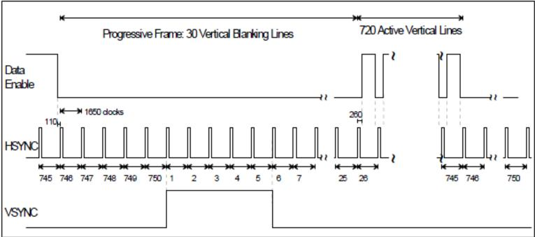
Figure 3. Timing parameters for 1280x720p @ 59.94/60 Hz.
