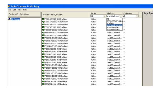
7. A list of available connections for the XDS100USB Emulator will appear in the middle of the Setup CCS screen, under "Available Factory Boards". Click on the configuration "F28027 XDS100 USB Emulator" and add to the "System Configuration" (left panel). The setup CCS window will then look like the following:
