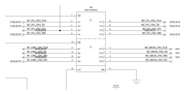
Second stage is the translator in question. – after this stage signals go directly to Virtex V6 no other connections.
