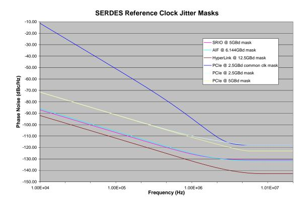
Since this graph will be difficult to use, we also provide this information as a straight-line approximation with the end points and the knee defined. This template is shown in the graph below and the endpoints in the table that follows. The mask level at specific frequencies can now be estimated based on the straight-line approximation. This is useful when comparing clock sources from various vendors who specify jitter masks in different ways.
