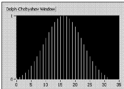
The  $s$  parameter adjusts the side lobe level of the Dolph-Chebyshev window. The lower the side lobe level, the wider the main lobe. The following front panel shows the fast Fourier transforms of Dolph-Chebyshev windows with  $s = 80, 100$  and  $120$  dB, respectively.
