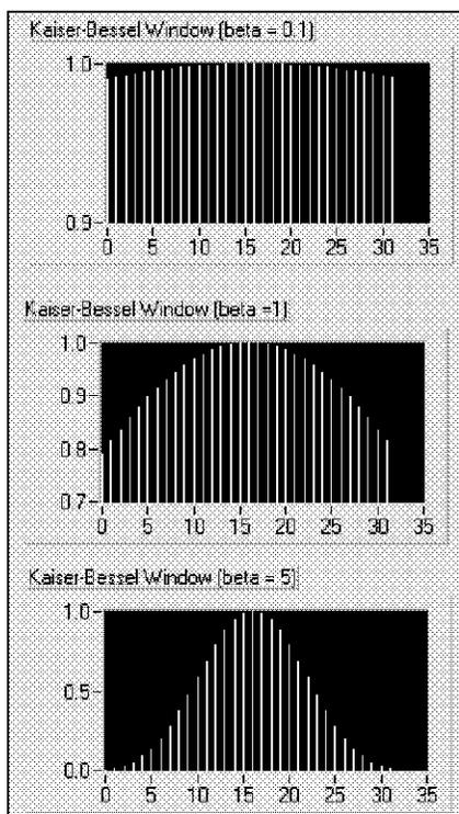
For small values of **beta**, the shape is close to that of a rectangular window. Actually, for **beta** = 0.0, you do get a rectangular window. As you increase **beta**, the window tapers off more to the sides.
