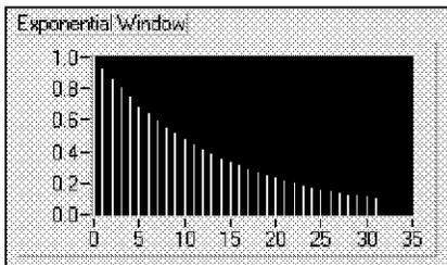
The exponential window is useful for analyzing transient response signals whose duration is longer than the length of the window. The exponential window damps the end of the signal, ensuring that the signal fully decays by the end of the sample block. You can apply the exponential window to signals that decay exponentially, such as the response of structures with light damping that are excited by an impact, such as the impact of a hammer.
