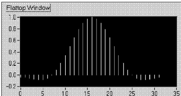
The flat top window is most useful in accurately measuring the amplitude of single frequency components with little nearby spectral energy in the signal.
