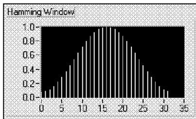
The Hanning and Hamming windows are similar, as shown in the previous two front panels. However, in the time domain, the Hamming window does not get as close to zero near the edges as does the Hanning window.
