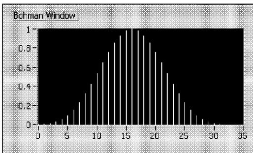
LabVIEW convolutes two sine lobes of half length to obtain the Bohman window. The following front panel shows the sine lobe.
