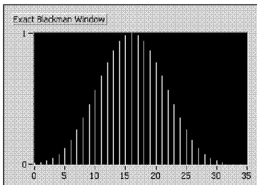
The Exact Blackman window is useful for single tone measurement. The Exact Blackman window has a lower main lobe width and a lower maximum side lobe level than the Blackman window. However, the Blackman window has a higher side lobe roll-off rate than the Exact Blackman window.
