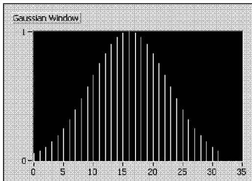
The Gaussian window is useful for time-frequency analysis because the Fourier transform and the derivative of a Gaussian window both are Gaussian functions. For example, a Short-Time Fourier Transform with a Gaussian window is the Gabor transform.
