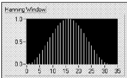
The Hanning window is useful for analyzing transients longer than the time duration of the window and for general-purpose applications.
