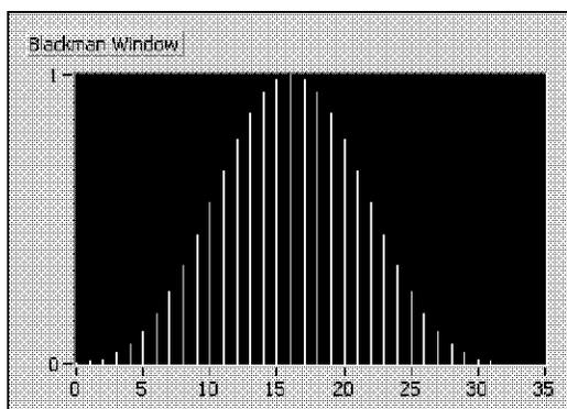
The Blackman window is useful for single tone measurement because it has a low maximum side lobe level and a high side lobe roll-off rate.
