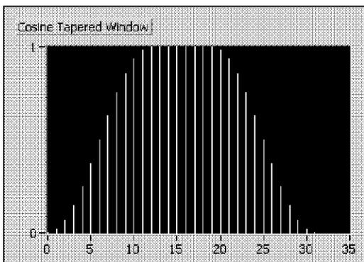
The cosine tapered window smoothly sets the data to zero at the boundaries without reducing significantly the processing gain of the windowed transform.
