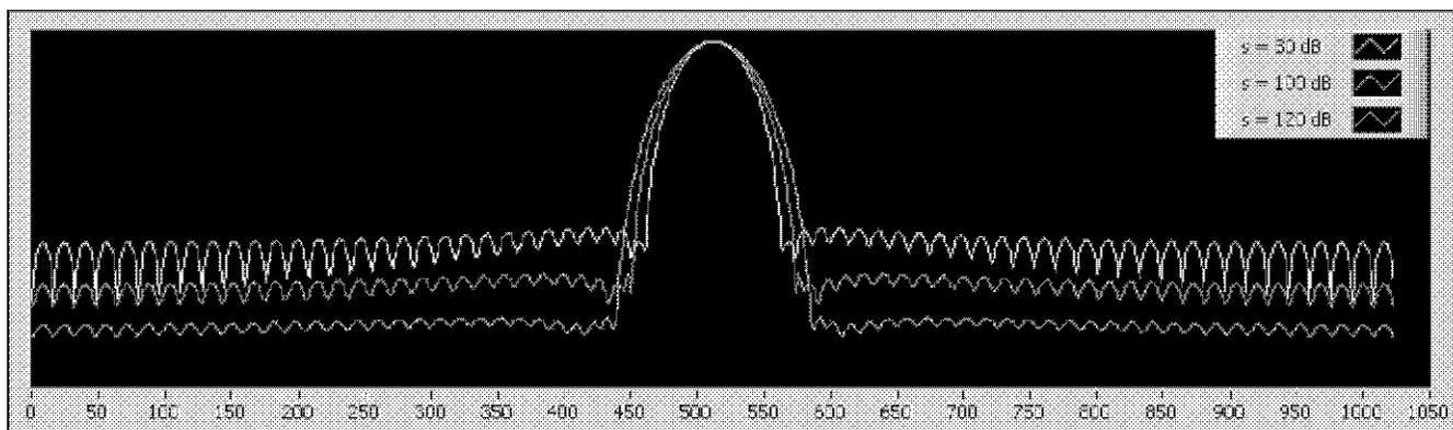
All side lobe levels of the symmetric Dolph-Chebyshev window have the same height, as shown in the following front panel.
