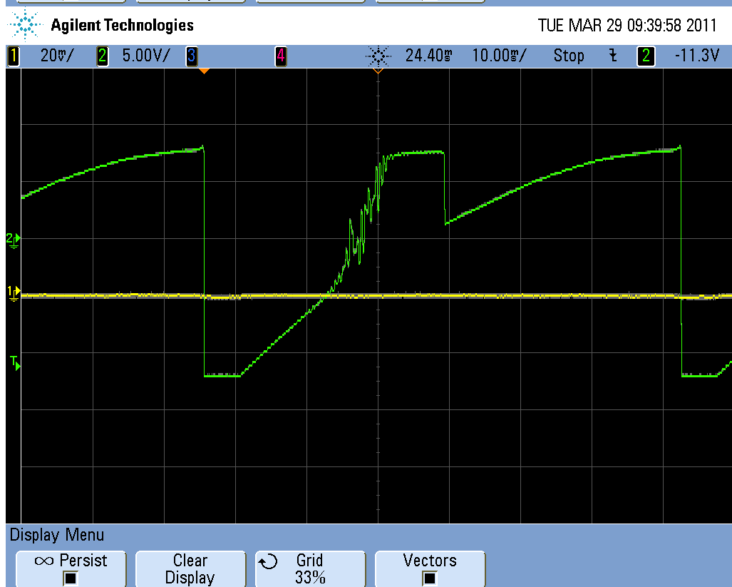
Figure 5. +12V (upper) and -12V (lower) during output signal period. AC mode 20mV/div. Infinity persistence.
