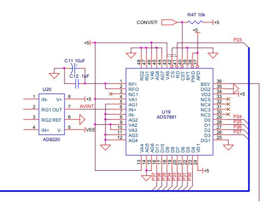
We have a problem reading data from this converter – we get all ones, which is the default state for the data bus because it has weak pull-ups. As you can see, CS! Is tied low, so that asserting RD! should put data on the bus, but apparently the chip disagrees. We know it is cycling because BY goes high during the conversion. Have I missed something here or should I look elsewhere?
