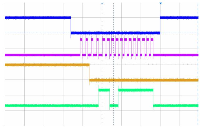
3. First Read Converted Data with Cmd 0xD and Read with 13 Clocks with Extra Bit for TAG Bit: Data Read = 0x180 (TAG 0 for Channel 0)
