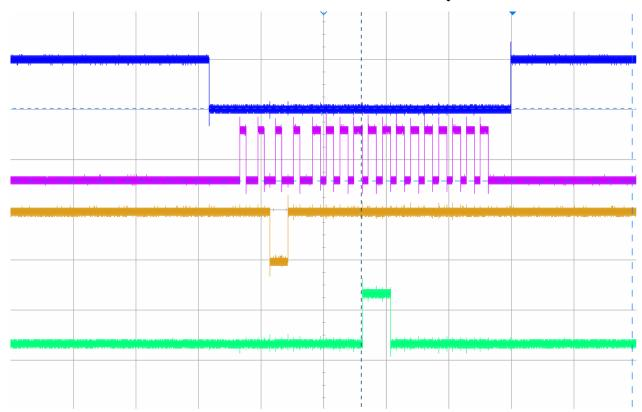
4. Second Read Converted Data with Cmd 0xD and Read with 13 Clocks with Extra Bit for TAG Bit: Data Read = 0x180 (TAG 0 for Channel 0): Same 1<sup>st</sup> Channel, Not the 2<sup>nd</sup> One
