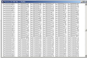
An inspection of the target devices memory shows that the data for the write to address 608 did not make it to memory. But the Gpp is moving to the next address This is a scope trace of the FRAME signal. The upper signal is only a trigger:
