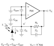
Figure 1. Transimpedance Circuit with Modeled Elements
