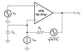
Figure 4. Noise Analysis Circuit
