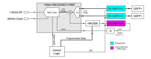
The Hittite ADC uses logic levels with a negative common-mode voltage. Connections to logic with a different common-mode voltage, eg., the TI retimer and Altera Stratix IV GT FPGA transceivers, requires AC-coupling and data modulation so that the serial data stream has no DC bias.
