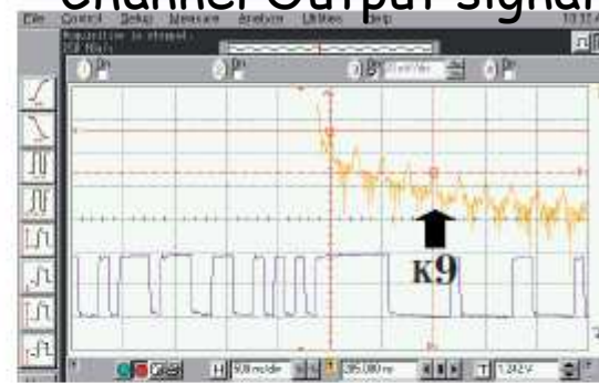
Figure 17: Output signal eye diagram, with de-emphasis
