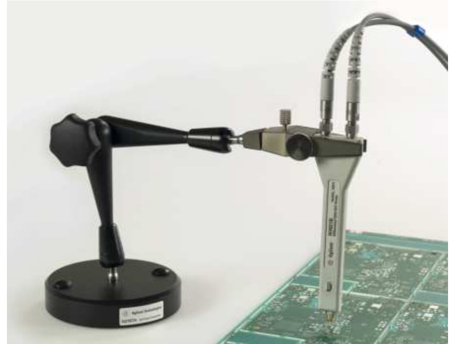
Agilent TDR Probe N1021B (100Ohm, 18GHz) mounted in 3D Probe Positioner N2787A could be used for pattern injection up to 18GHz.
