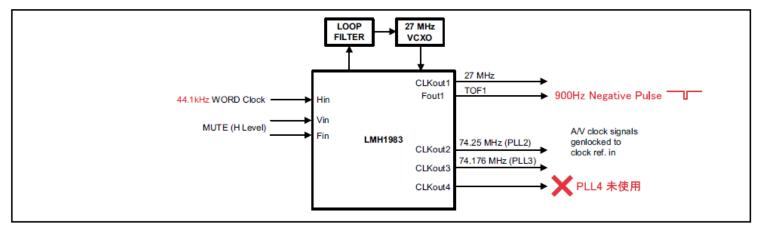
Negative Pulse of 900Hz cycle is outputted from Fout1 terminal. common denominator (27 MHz and 44.1 kHz), it is guessed that the phase comparison frequency of PLL1 is 900Hz. Reference lock time: About 30 seconds
