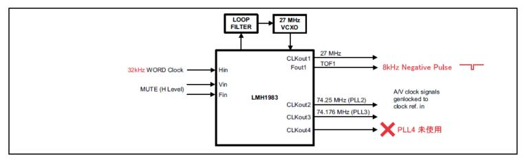
Negative Pulse of 8Khz cycle is outputted from Fout1 terminal. common denominator (27 MHz and 32 kHz), it is guessed that the phase comparison frequency of PLL1 is 8 kHz. Reference lock time: About 6 seconds
