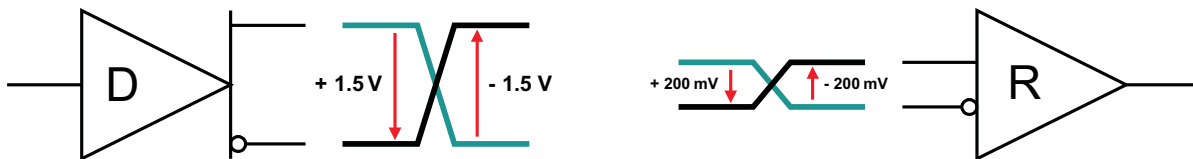
Figure 3. RS-485 Specified Minimum Bus Signal Levels
