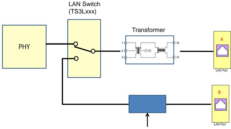
May need Transformer to isolate LAN switch and LAN port
