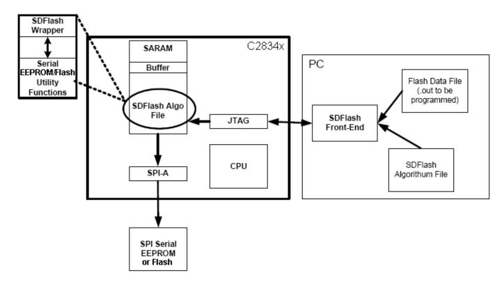
The flash data file is first prepared to include the header information required by the on-chip SPI bootloader. With this information included, the "boot to SPI" option can then be used to copy the application into the 2834x device at boot time. Detailed information on the SPI boot header and the 2834x boot mode options can be found in *TMS320x2834x Delfino Boot ROM Reference Guide* (sprufn5) available on TI's website.
