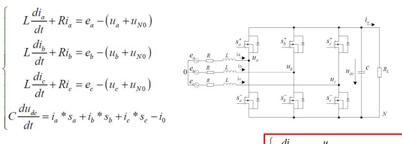
$s_k = \begin{cases} 1, & \text{up switch closed, down switch opened} \\ 0, & \text{up switch opened, down switch closed} \end{cases}$
