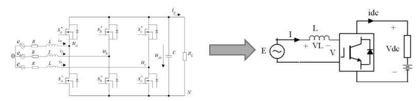
The PWM Rectifier can be equivalent to the figure above, then we can get the the equation:
