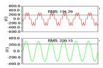
It is a non-controllable rectifier, the input current contains many harmonic waves. (ie, 5,7,11,13....)
