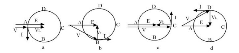
When the V trace from the A to B in the above figure, the converter can work in rectifier mode, when the V at the B, then the we can get the highest power factor.
