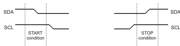
Figure 24-3. START and STOP Conditions
