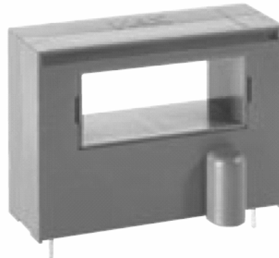
Fig 8 Example of a passive current sensing module (100 A rms , ± 160 A peak ), offering a large window (26 x 11 mm) in a compact housing (approx. 40 x 30 x 14 mm)
