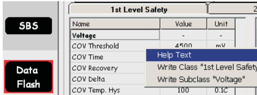
Figure A-2. Using bqEVSW Help System With bq20z80 v1.02 Device
