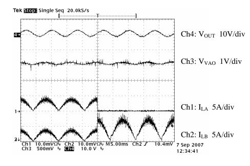
With immediate compensation of the R<sub>IMO</sub> value, virtually no disturbance occurs on V<sub>OUT</sub> and the VAO output is also undisturbed.
