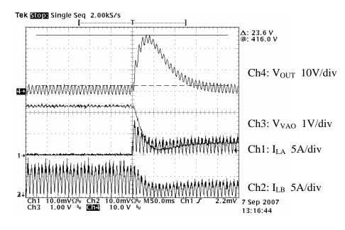
A ~24V overshoot occurs on V<sub>OUT</sub> because of the slow voltage-loop response of the voltage error amplifier when a phase is added.
