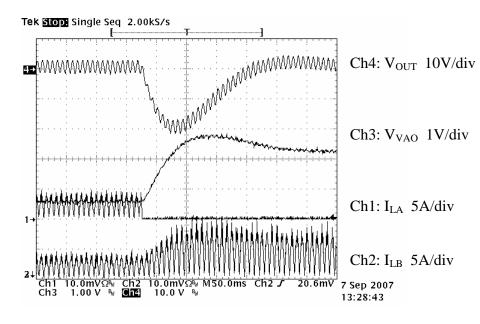
A  $\sim$ 20V droop occurs on V<sub>OUT</sub> because of the slow voltage-loop response of the voltage error amplifier when a phase is dropped.
