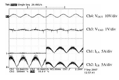
With immediate compensation of the  $R_{IMO}$  value, virtually no disturbance occurs on  $V_{OUT}$  and the VAO output is also undisturbed.
