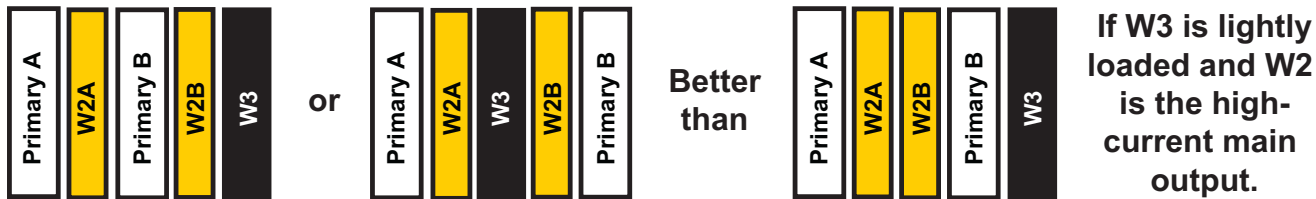
Fig. 8. Winding placement can affect leakage.
