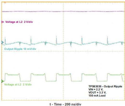
The Ripple waveform of TPS63030EVM-417
