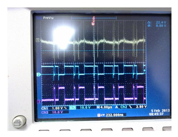
CH1 – Output Ripple CH2 – High Switch
