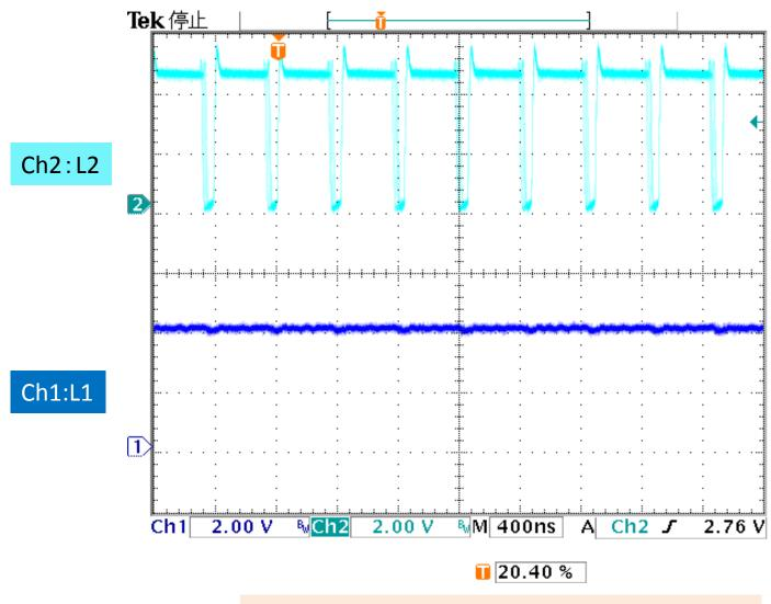
This wave form is in the Boost Mode. L1 pin is permanently High in the Boost Mode.
