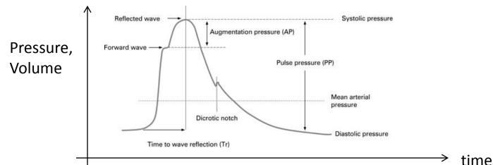
The above picture is waveform of pressure over time.
