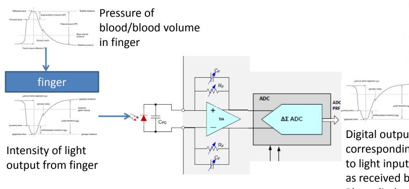
Digital output corresponding to light input as received by Photodiode
