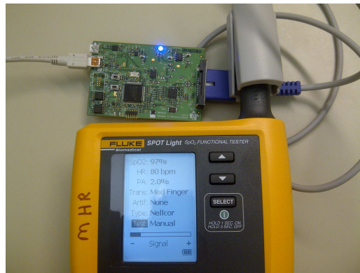
Figure 35. Fluke SPOT Light SpO2 Functional Tester Setup
