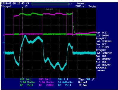
Mechanism pushed off from static demended positin. Ch 4 Phase A motor winding current @ 5mA/Div
