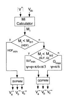
Fig. 13. The combined high-performance PWM algorithm flow diagram.
