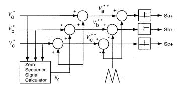
Fig. 2. Triangle-intersection-technique-based PWM employing the zero-sequence injection principle.
