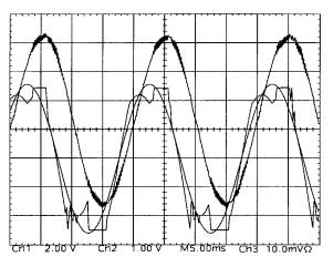
Fig. 16. Transition from SVPWM to GDPWM ( $M_i = 0.81$ , 50 Hz, 50%  $T_{eR}$ ) with  $\psi = \varphi + 30^\circ \le 60^\circ$ . Scaling: 2 A/div, 2 V/div, and 5 ms/div.
