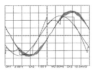
Fig. 17. Experimental GDPWM modulation wave, its fundamental component, and the motor current waveforms ( $M_i = 0.82, 51$  Hz, 50%  $T_{eR}$ ) with  $\psi = \varphi + 30^\circ \le 60^\circ$ . Scaling: 2 A/div, 2 V/div, and 2 ms/div.
