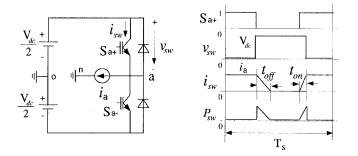
Fig. 8. PWM-VSI single-phase model for commutation analysis and per-carrier-cycle switching loss diagram under linear commutation.
