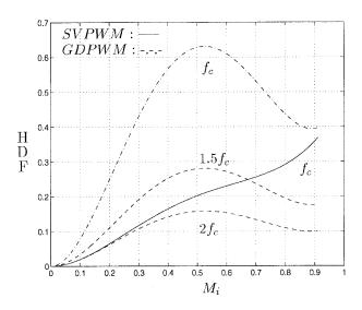
Fig. 14. HDF =  $f(M_i)$  curves of SVPWM and GDPWM for various carrier frequency values illustrate the optimal transition points/regions.
