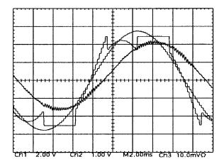
Fig. 18. Experimental GDPWM modulation wave, its fundamental component, and the motor current waveforms ( $M_i = 0.854, 53$  Hz, 100%  $T_{eR}$ ) with  $\psi = \varphi + 30^\circ \le 60^\circ$ . Scaling: 5 A/div, 2 V/div, and 2 ms/div.
