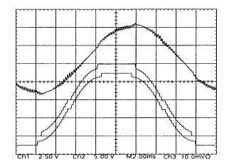
Fig. 24. GDPWM modulation wave, PEM-controlled modulation wave, and the motor current waveforms for  $M_i = 0.867, 53$  Hz with  $\psi = 30^{\circ}$ . Scaling: 5 A /div, 2 V/div, and 2 ms/div.
