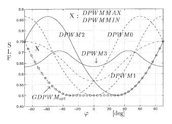
Fig. 11. SLF =  $f(\varphi)$  characteristics of the modern DPWM methods under fixed carrier frequency constraint (SLF<sub>CPWM</sub> = 1).
