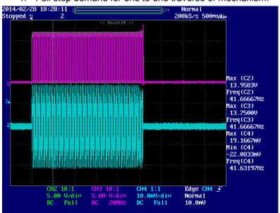
2. Expanded view of drive demand / winding current
