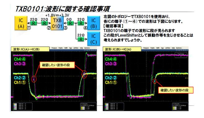
Change resistor  $0\Omega$  to  $22\Omega$ .
