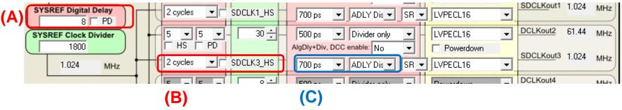
The best way to adjust SYSREF to Device Clock setup-hold time is with SYSREF operating in continuous mode.
