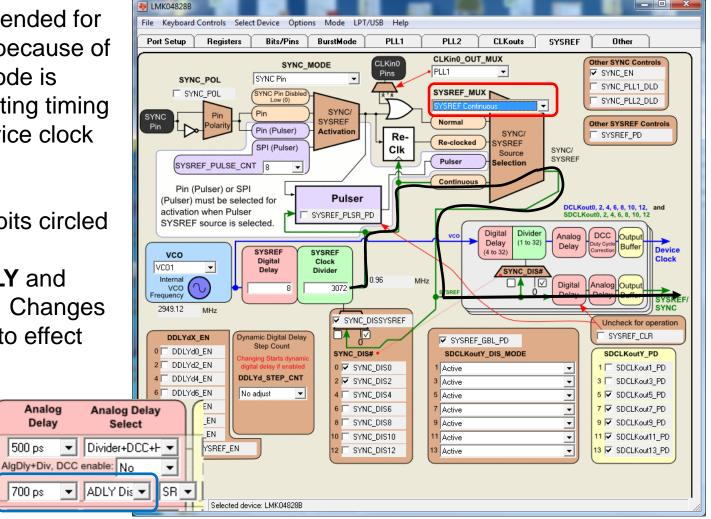
Analog delay (blue box) has +/- 30% variation over PVT. It is best to use analog delay only with slower device clock frequencies.
