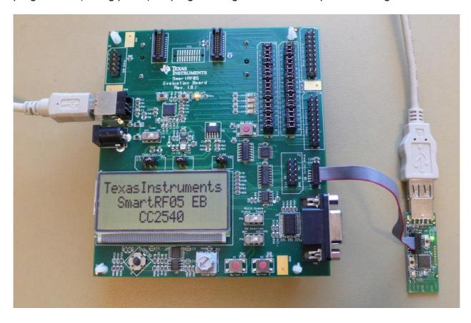
Note the orientation of pin 1 (red wire) on the debug cable and that the dongle is connected to a USB port (required for powering the device).
