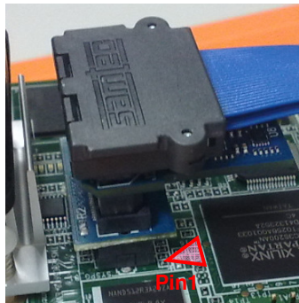
Figure22: The connection with TI XDS560v2 STM Emulator
