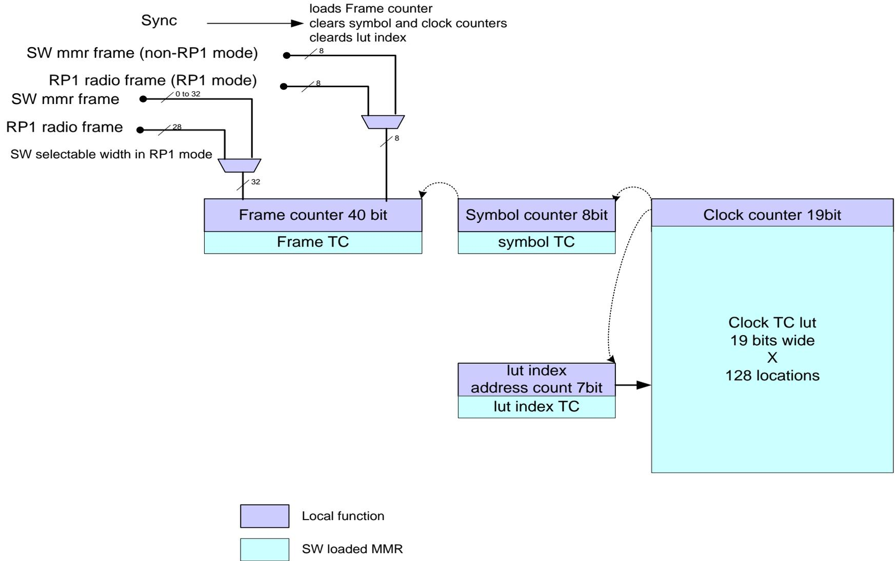
lut index address terminal counter is used for various size of symbols.
