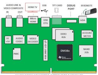
244 PIN SODIM CONNECTOR INTERFACE TO BASE BOARD
