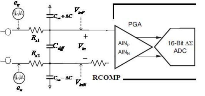
\*As long as C<sub>diff</sub> ≥ 10\*C<sub>cm</sub>, mismatch in C<sub>cm</sub> (△C) will be attenuated to insignificant levels
