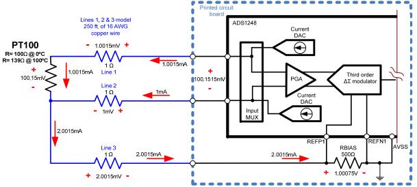
For the three-wire setup for an RTD measurement, advantages are:
