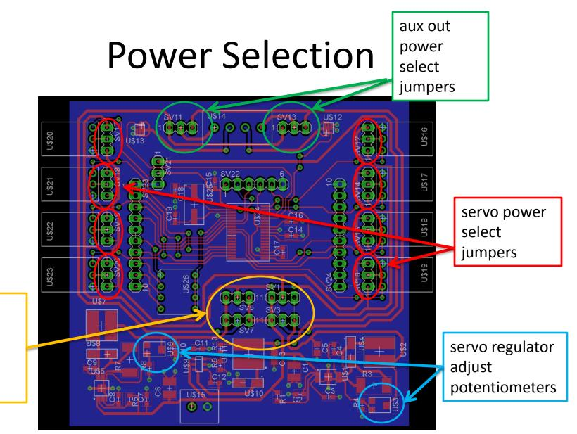
servo and aux out regulator bypass jumpers
