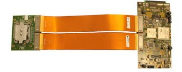
The VX4100 Board supports the largest DMDs with 0.95" and 0.96" diagonal array size, respectively. The control and data lines for the 2xLVDS DMD are put into two flexible cables of 5" or 12" length giving a high degree of freedom for the optical arrangement.
