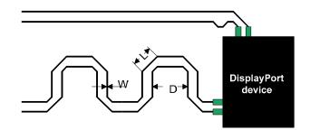
Fig. 7. Skew reduction via meandering using chamfered corners
