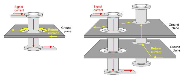
Fig. 14. Return current paths for a single- and a multiple layer change
