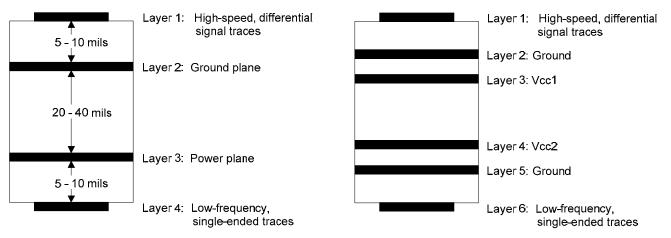
Fig. 2. Recommended 4- or 6- layer (0.062") stack for a receiver PCB design
