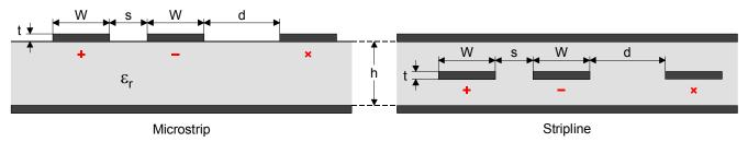
Fig. 5. Physical geometries of differential traces
