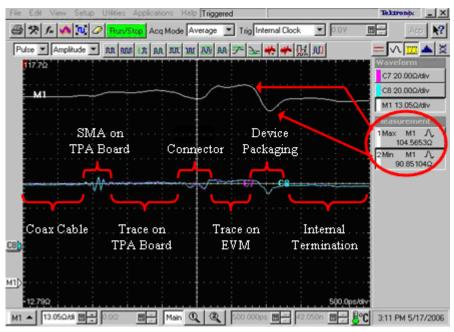
Fig. 6. TDR display revealing the locations of discontinuities
