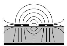
Fig. 12. Field coupling within a microstrip structure
