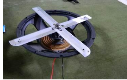
Figure 12 –Tactile transducer for seat mounting.
