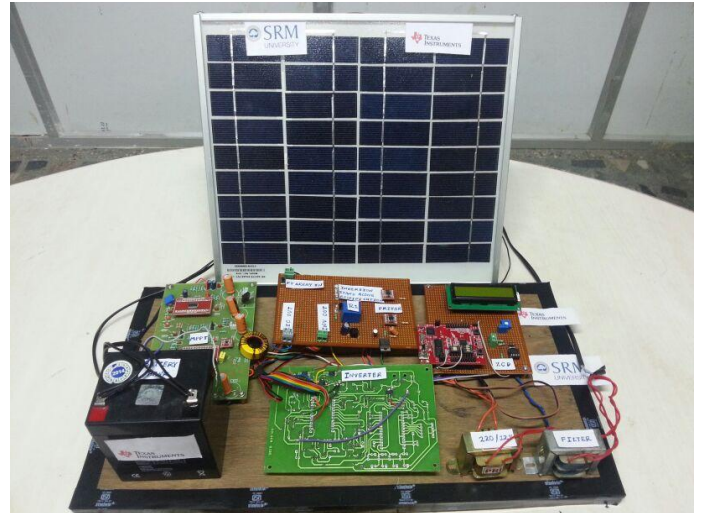
Figure 3.3: Hardware implementation of the HUB
