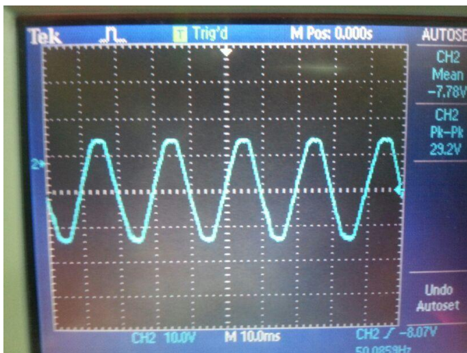
Figure 4.5 : Filtered output sin wave of the inverter
