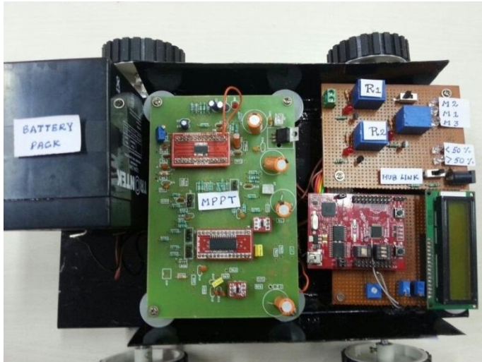
Figure 3.2: hardware implementation of the vehicle
