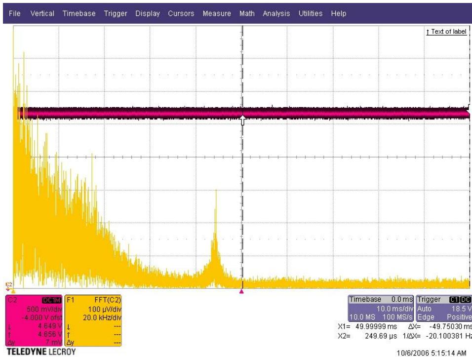
On the first picture, you can see the photo diode voltage and the FFT of this voltage by using the EvalBrd. There is almost no noise between a frequency of 0 and 100kHz. Just a peak of 150uV by 38kHz, which is also existing, if the LED is turned off. (look at "HeliSorce SC1 Evaluation of the TI LM3409")
