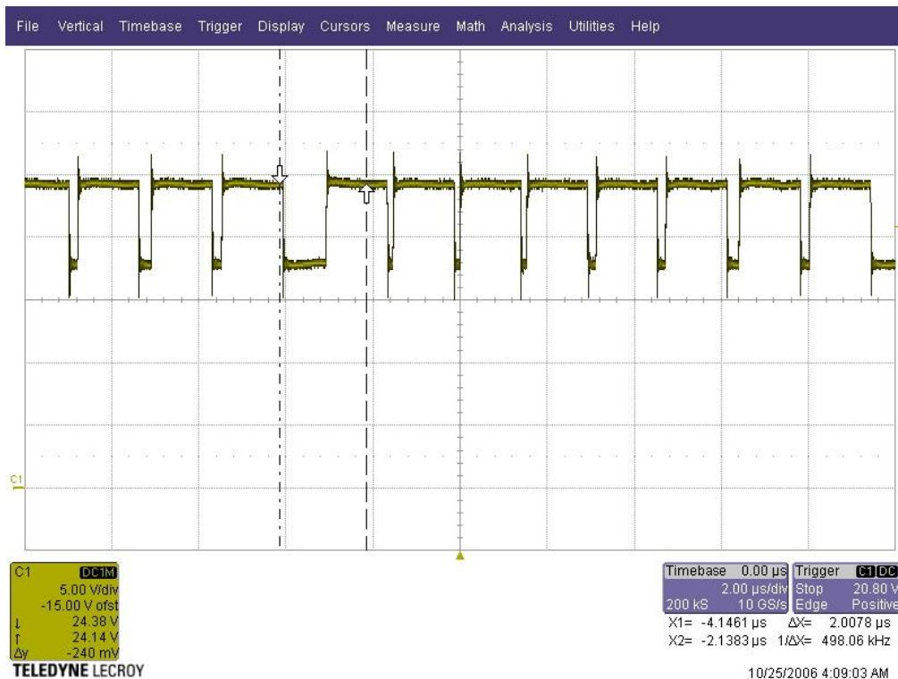
On the first picture, you see the switching behavior of the PGATE on the Evaluation Board. The High signal (24V) is equal to the Off time, which is adjusted by COFF. During the Low signal (17.5V), the FET (Q1) is conductive. This duty cycle is almost constant.
