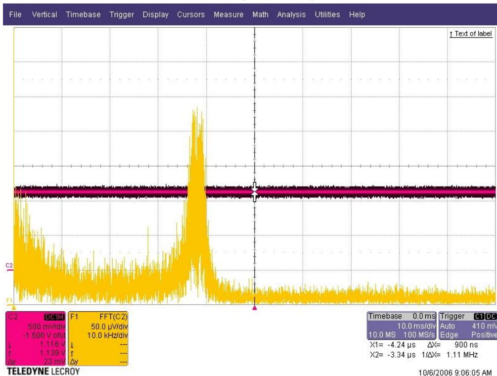
If  $I_{LED} = 2A$ , the problem is still the same. There is much noise between 0-and 50kHz (factor 2-3 comparing to EvalBrd). The peak at 40kHz doesn't exist on the EvalBrd.
