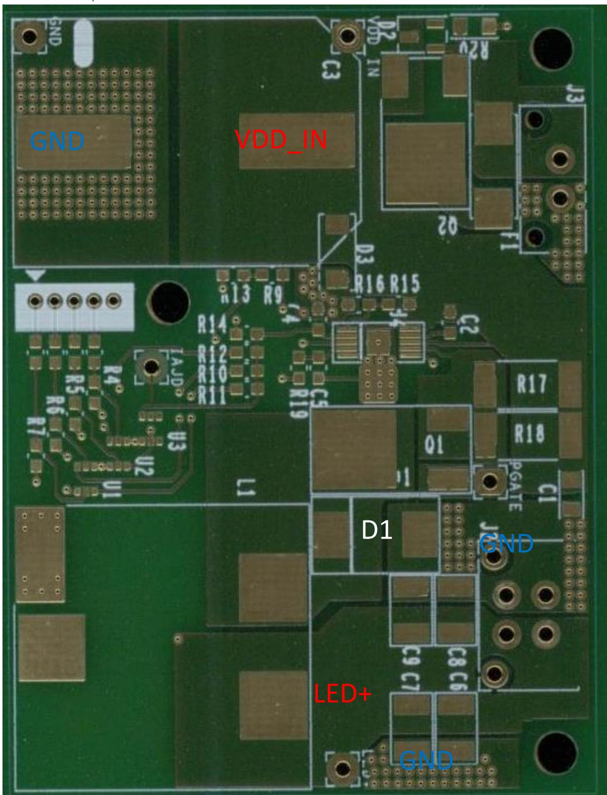
The components on the HeliSource and the Evaluation Board are identical, especially the schottky diode D1, the inductivity L2 and the FET Q1.
