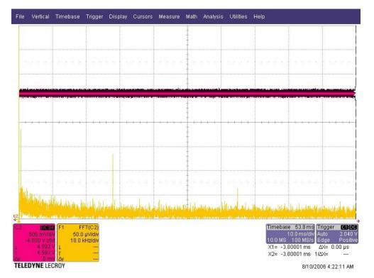
The first picture shows the noise between 0 and 100kHz, when  $V_{IN}$  is 24V. The second picture shows the noise between 0 and 100kHz, when  $V_{IN}$  is 12V. If you compare the amplitude of this noises, you
