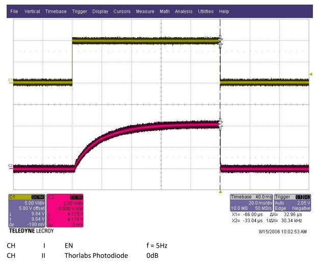
On this picture, you can see, that after 80ms the voltage generated by the Photodiode, cause of the light, produced by the LED, is constant. This means, that the LED current is constant as well and the system is ready for measurement.
