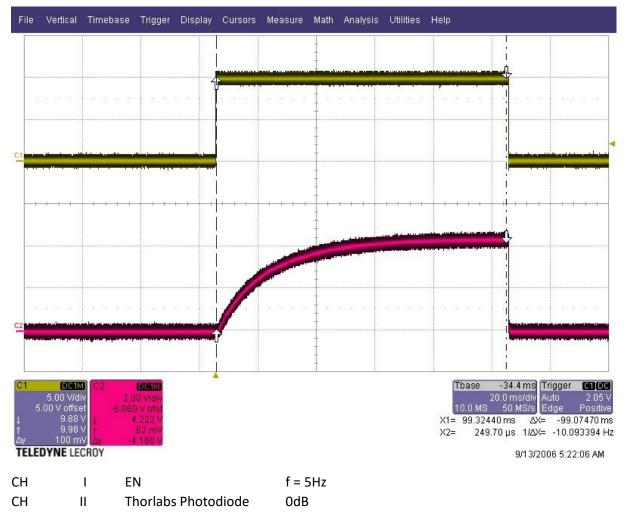
For this measurement, the setup was modified with a 2.2kOhm resister between Vin and LED+. So a DC Offset of 2.3V was generated. Unfortunately there was no positive effect on the Current rise time.
