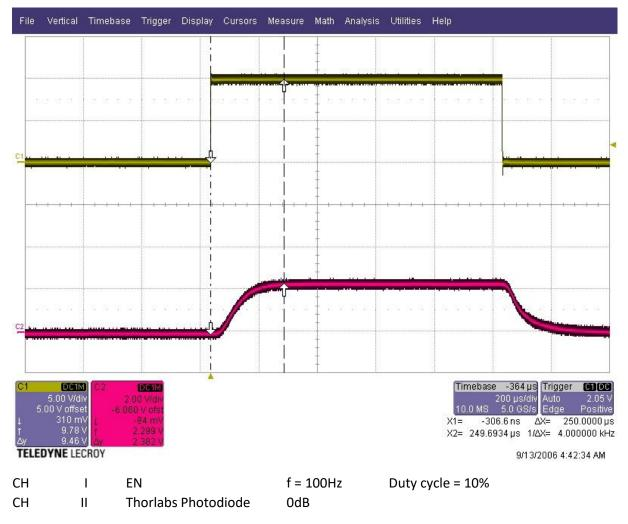
On this picture, you can see, if the frequency on EN is 100 Hz with a Duty cycle of 10%, the current rising delay is only 250us. This is a factor 400 faster.
