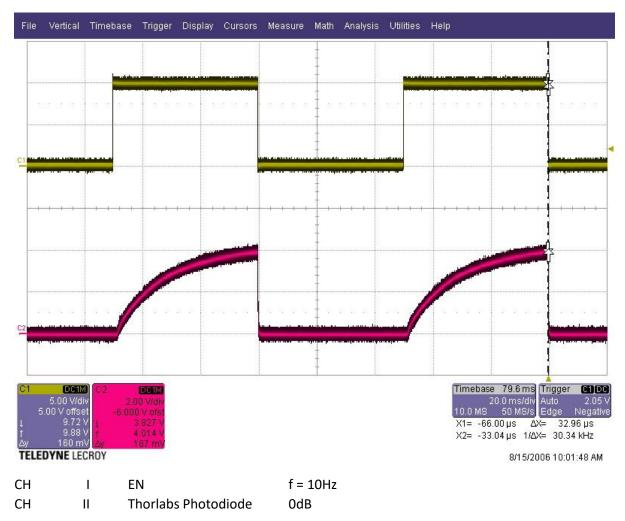
On this picture, you can see, that the voltage generated by the Photodiode, cause of the light, produced by the LED, is still rising, when the EN is set to GND, and the device is turned off. This means, that the HeliSource isn't started up and not ready to make any measurements by constant LED current.
