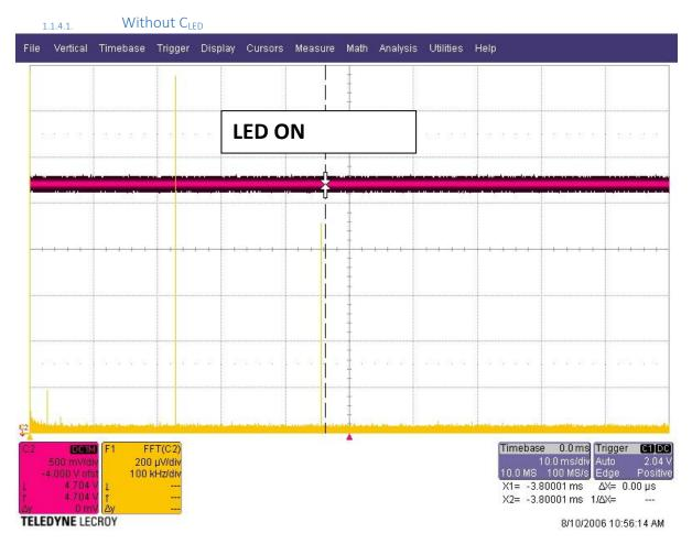
If the capacitor between anode and cathode of the LED is removed, the amplitude noise on 220khz is about 1.6mV instead of 150uV. This means the noise/signal ratio is about factor 10 bigger. In addition to, a new noise at 460kHz is measured. The amplitude of this noise is about 900uV.
