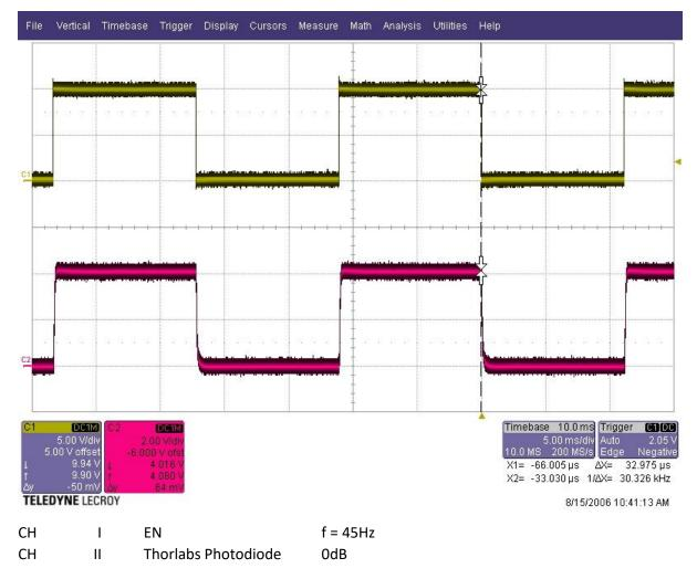
On this picture, you can see, if the frequency on EN is rising to 45Hz or higher, the rise time of the LED current (proportional to V Photodiode) is reduced. This means, that the system is faster ready for measure when the frequency at EN is 45Hz or higher.
