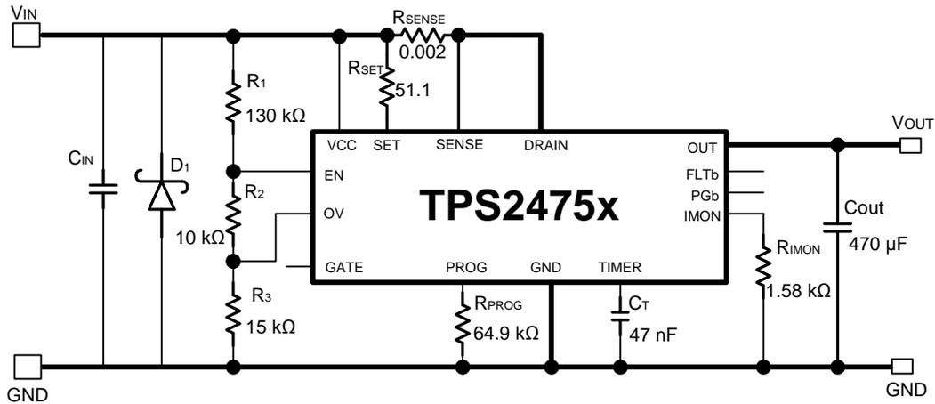
Figure 1. TPSD2475x as the 12-V, 10-A eFuse
