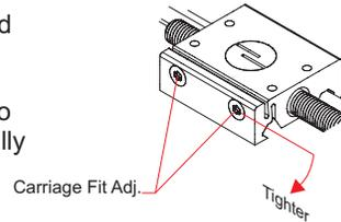
**!** Over tensioning carriage will result in binding, rapid lead screw, nut, and pad wear.
