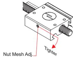
**!** A squealing lead screw/nut is an indicator that adjustment or lubrication is needed
