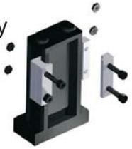
1. Set the gusset and Z axis on the carriage of the X axis. See sketch at right. Insert four XMB-2 bolts (6-32 x 1/2" socket head cap) but **do not tighten**. Fasten gusset to base of Z axis with supplied cleats/bolts/nuts, tighten **finger tight only**.
