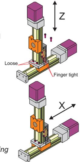
*Thread locking compound (Loctite) is recommended for all mounting bolts.*
