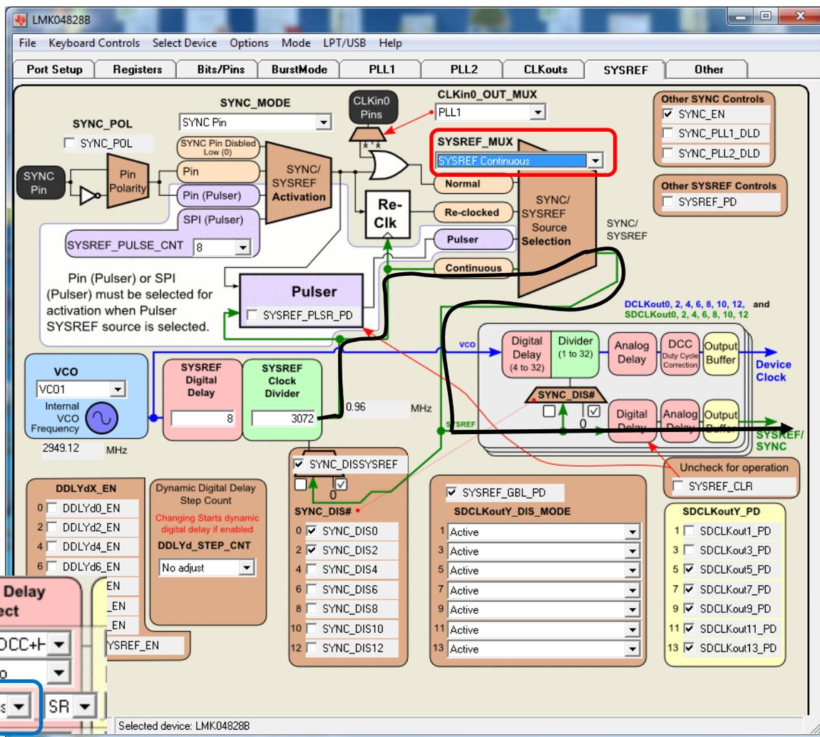
Analog delay (blue box) has +/- 30% variation over PVT. It is best to use analog delay only with slower device clock frequencies.
