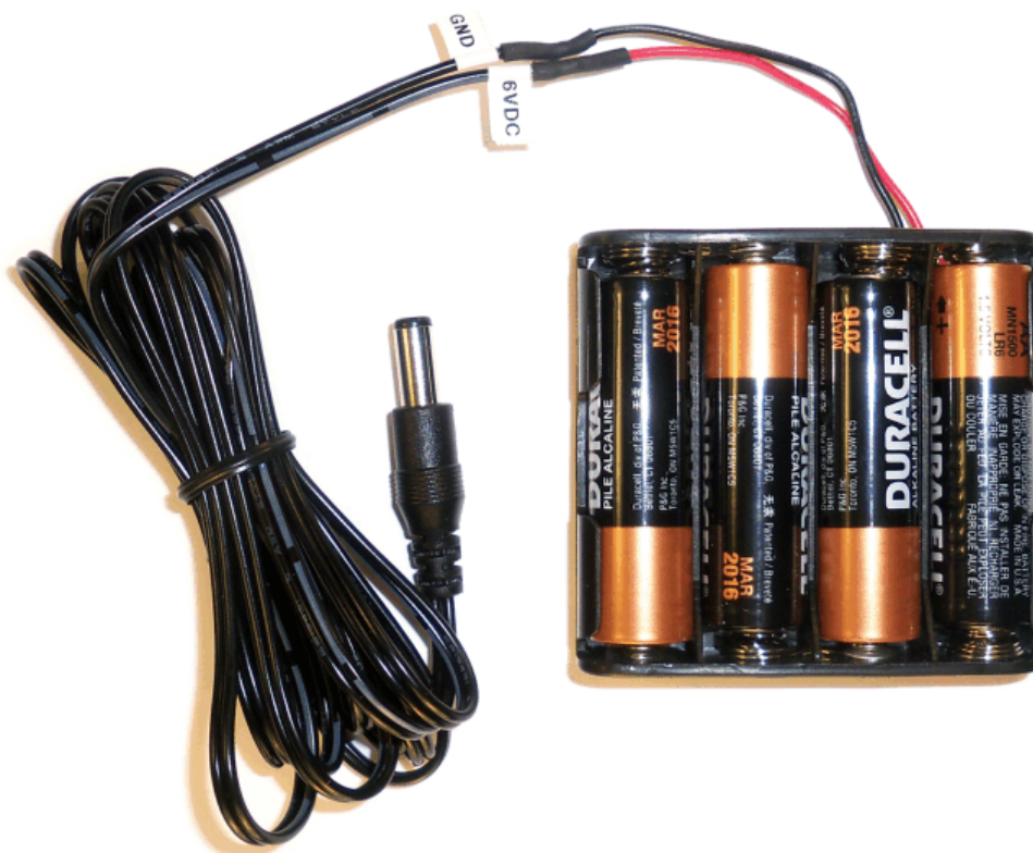
Figure 71. Recommended Power Supply for ADS1298ECG-FE
