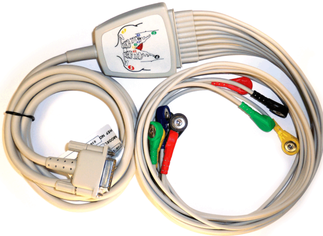
Figure 67. 15-Pin, Shielded Connector from Biometric Cables
