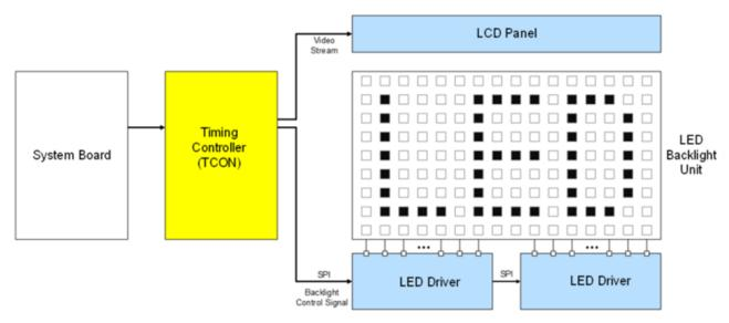
Figure 2. The components of a local dimming system for automotive displays
